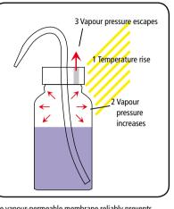
The vapour-permeable membrane reliably prevents leaking of the contents when temperatures rise.
