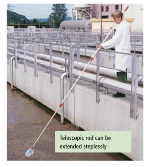
Versatile sampling system with exchangeable tools for a wide range of applications.
