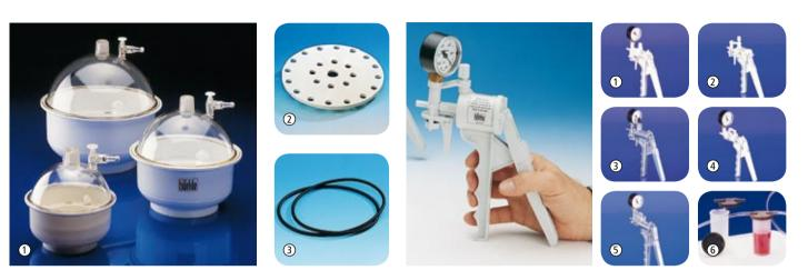
Plastic desiccators are unbreakable and lightweight – two essential advantages! With stopcock, for vacuums up to 980 mbar. Base and desiccator plate are made out of polypropylene, the lid is crystal-clear polycarbonate with both a non-return valve and a venting valve. O-ring seal made of polychlorobutadiene-rubber. 60 °C max. continuous temperature.
