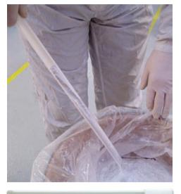
The disposable PowderDispo is ideal for taking a cross sectional sample from within a bulk powder.
