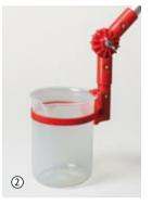
② Angular beaker Adaptable to different container shapes by adjustable angle setting (up to 90°).
