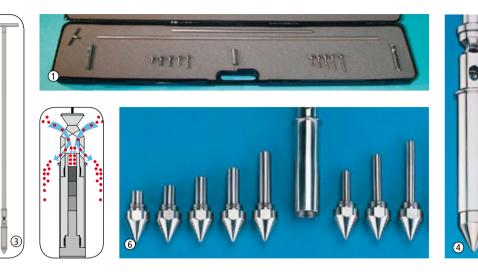
PharmaPicker has been developed specially for sampling very small quantities of highly potent, expensive or active powders. Different tip container volumes from 0.1 to 2.5 ml (see table) can be replaced simply and quickly. PharmaPicker is made of AISI 316 stainless steel and is electropolished, thereby complying to GMP guidelines. All parts can be easily cleaned and disassembled. Note: Capacity tips have to be ordered separately!
