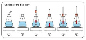
Magnetic stirrer is not supplied with fish-clip<sup>®</sup> Suitable Magnetic stirring bars you can find on page 178. With fish-clip<sup>®</sup> cell cultures, abrasive media and other liquids that are sensitive to mechanical stress are gently stirred. No disruption of biocatalysts such as enzymes or cells. No scratching the vessel base, no broken vessels resulting from stirrer bars "jumping about".
