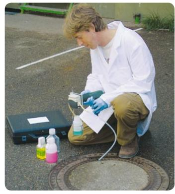
Vampire in use in the environmental protection sector for sampling from narrow openings and at substantial depths.
