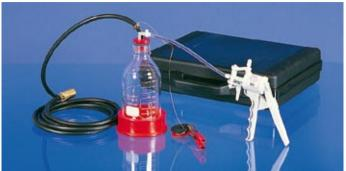
Developed for sampling flammable liquids of hazardous materials VbF Hazard Class AI (VbF is the German Regulation concerning Flammable Liquids). Glass bottle and hose are connected in such a way that they conduct electricity and are grounded via a grounding cable.
