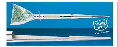
StickProof sampler for powders in the pharmaceutical industry, made of AISI 316 stainless steel. The especially slender tip can be inserted easily and deeply. The conical inlet of the tip lets you collect either very small or larger quantities. StickProof is constructed in one piece without edges, grooves or crevices for perfect and easy cleaning. The sample can be filled directly into the sampling bag. Fasten the bag with a sturdy clamp.
