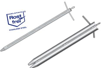
For viscous substances like pastes, muds, creams, oils. Made of AISI 316 stainless steel, electropolished and ideal for use in pharmaceutical areas. The sample is drawn in using the pump rod and directly conveyed to the sampling container. Easy cleaning for flawless sampling. Suction capacity 30 ml to 75 ml. Depending on the viscosity, the unscrewable suction head can be fitted with suction drills of 2 mm to 6 mm.
