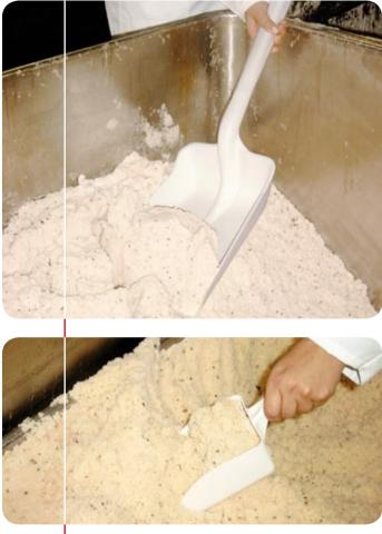
Iron scoops are loud, can be dented and rust and are also heavy. Plastic scoops have none of these disadvantages and are also hygienic, because they are made in one piece and have a non-stick surface. They also have a high chemical resistance, are unbreakable and, depending on the version, may be anti-static, anti-microbial, suitable for use with food and available in different colors (cadmium-free) – all valuable advantages.
