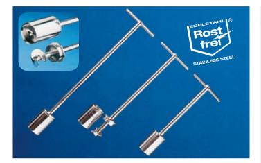
Developed for sampling from frozen, high viscous, pasty materials and similar substances. The Ice-Sampler screws into the sample material and simultaneously extracts and conveys the sample into the sampling cylinder. The sampling cylinder is detachable.
