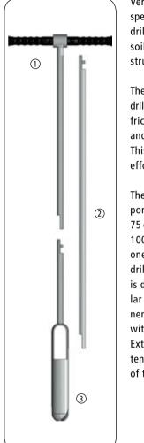
Very robust model with specially hardened forged drill bits. For determining soil properties, moisture, structure.
