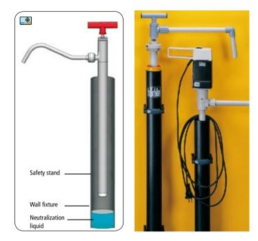
Safety stand for pumps protects against leaking chemicals Filled to one third with the appropriate neutralization agent or water, any residual liquid from the pump is diluted, neutralized and rendered safe.
