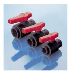
Made of fibre-glass reinforced PP, red handle with Viton and PTFE O-rings, maximum pressure 10 bar (at  $+ 20 \degree$ C), maximum temperature + 100 °C.
