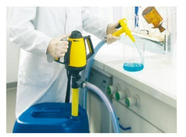
Low weight pumps with high delivery output for the transfer of small quantities of liquids with a viscosity up to 300 mPas from canisters, drums and narrow-necked vessels with a diameter from the mouth from 25 mm upwards.
