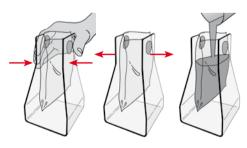
Adhere sticky putty, insert bag into open BagOpen, squeeze BagOpen – release – fill sample bag
