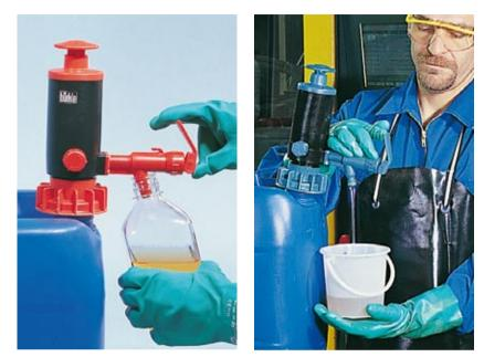
PumpMaster container pumps are designed for fast and clean emptying of canisters and small barrels. Excess pressure is generated using the piston handpump, which pushes the liquid out of the container. Pump capacity approx. 9 l/min. The sensitive discharge control valve allows even small amounts of liquid to be discharged.
