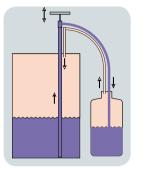
Liquid is pumped in a closed system (blue). Vapors are returned to the container via the gas-shuttle pipe (pink).
