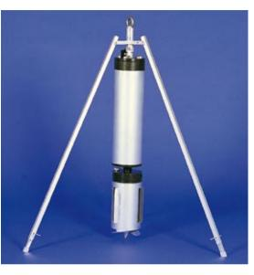
It is often very difficult to take a sample from a partly filled silo. Sampling with a beaker on the end of a long rod is not only wearisome and time consuming, it is sometimes impossible to obtain a sample. Eagle works semi-automatically and can be used down to a depth of 10 m without any problems. The support legs are fold up so that Eagle can access the silo contents through openings that are only 150 x 150 mm.
