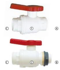
New - now also for foodstuff, made of fibre-glass reinforced PP, ball made of PP-G, handle with O-ring NBR, seal HDPE. Max. pressure 10 bar (at + 20 °C), max. temperature 100 °C. Inner thread
