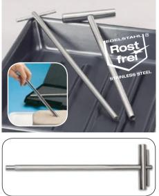
Cylindrical hollow drill with a sharp cutting edge. The hand-drill can easily be driven into paste-like and semi-solid substances by a rotating movement. The samples cut out are subsequently removed from the drill using the push-rod ejector. Drilling depth 20 cm, total length 260 mm, weight 386 g. Inside diameter 8 mm, Outside diameter 10 mm.
