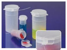
The sample tubes are produced under clean room conditions and formed at over 100 °C in the injection molding machine, so that the insides of the tubes are virtually sterile. This method makes the tubes absolutely leakproof, as the cap and tube adapt optimally to each other during the cooling process. Undercut-free, so easy to fill and can be emptied completely.
