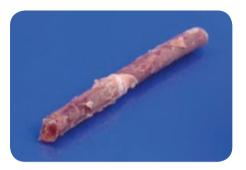
For deep-frozen products in the food industry and semi-solid substances. The sharp sawing crown of the very robust hollow borer rapidly cuts into the sample. A cylindrical sample (cross-sectional sample) with a diameter of 18 mm and a length of up to 20 cm can be cut out. Consists of three parts: borer, borer head for use in conventional drills and rod for pressing the cylindrical sample out of the borer head.
