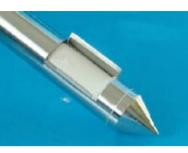
Scratcher has been developed specially for sampling of cohesive, caking, nonflowing substances.
