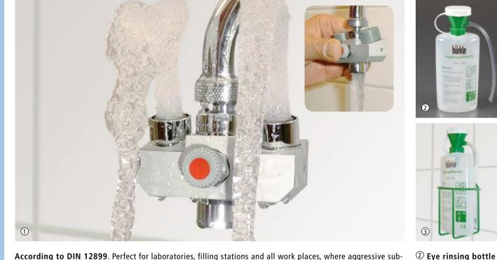
According to DIN 12899. Perfect for laboratories, filling stations and all work places, where aggressive substances are used. EyesFresh delivers streams of cold water immediately upon opening the tap. For normal use of the tap, just press the button. Afterwards, EyesFresh returns automatically to eyewash-function. Eyes Fresh can be fitted onto all cold water taps with ½" thread (outer thread M22x1) without extra installation work.
