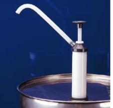
The piston pump is made of polypropylene and polyethylene, for aquous and petrochemical products. It offers a good price/performance ratio. The piston pump is attached to the container with a 2" or <sup>3</sup>/<sub>4</sub>" internal thread connection. After mounting it can still be rotated about its axis so that containers can be placed on the drum lid and filled.
