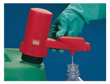
Pump-it canister pumps are designed for emptying canisters and small barrels up to 60 I rapidly and cleanly. The hand pump is used to create an overpressure that forces the liquid out of the canister.
