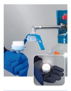
SnowPack<sup>®</sup> enables you to obtain a - 79 °C dry ice tablet weighing 50 or 250 g within a few moments, without complicated technology and without electricity! You can therefore obtain low-cost cooling to very low temperatures at any time you like. SnowPack<sup>®</sup> is often used in hospitals, universities, schools, institutes, laboratories, in the chemical industry and in materials testing facilities.
