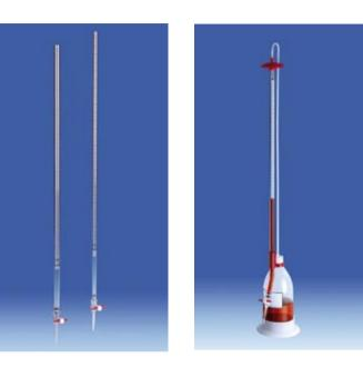
Schilling titration apparatus, consisting of plastic-coated buret made of borosilicate glass 3.3, class B (tolerances as per DIN ISO 385), with Schellbach stripe and high-contrast black printing. Adjusted for Ex. LDPE storage bottle with HDPE base and PP immersion tube.
