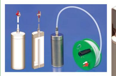
With the Target immersion cylinder, liquid samples can be taken from a particular point. The immersion cylinder is lowered on a strong and sealed tube. When the target has been reached, a valve at the tube end is opened; this vents the immersion cylinder and fills it with the sample. The immersion cylinder is pulled up and emptied via the screw thread.
