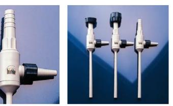
For withdrawing liquids and gases, and for creating vacuums; simple operation and easy cleaning. The vacuum connection can be unscrewed and a variety of water inlet connections (R  $\frac{3}{4}$ " sleeve nut, R  $\frac{1}{2}$ " reducing adapter and 10 – 12 mm o.d. tubing nozzle) simplify connection to most water sources.
