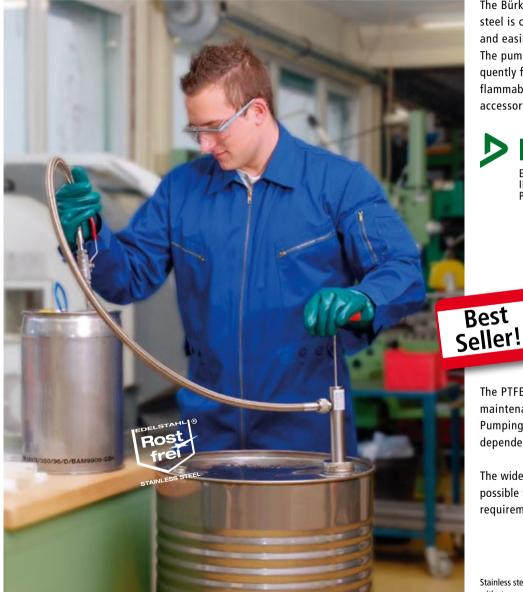
The Bürkle barrel pump made of stainless steel is constructed for filling combustible and easily inflammable liquids. The pump can conduct electricity and consequently fulfills the requirements for handling flammable liquids in combination with the accessory antistatic set.
