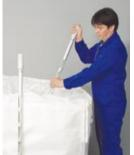
Ensures accurate zone sampling from all layers of the bulk goods. The spiral arrangement of the sampling slits means that these are opened one after the other from bottom to top. In this way the lowest opening is filled first and then those above it in sequence until the complete Spiralus has been
