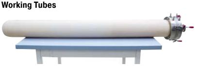
Working tube closed at one end with gastight flanges as additional equipment
