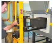
Working with protective gas boxes for a protective gas atmosphere using a loading carriage
