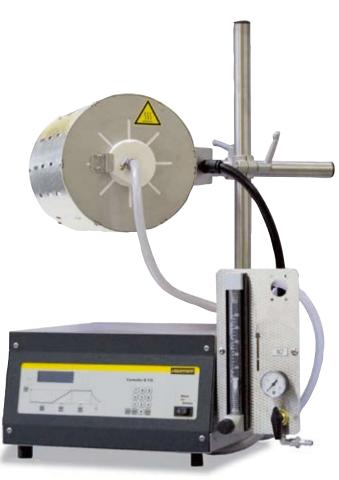
RT 50-250/11 with gas supply system for nitrogen
