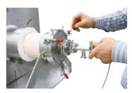
Water-cooled end flange with quick connectors as additional equipment
