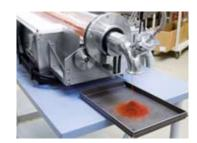
Protective gas inlet at tube exit
