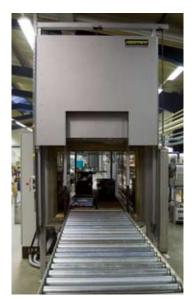
N 1680/45 AS with roller conveyor implemented in a production line
