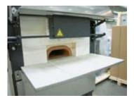
Work platform in front of muffle to place load
