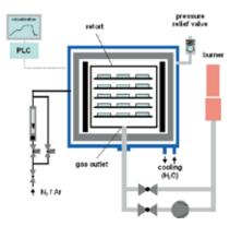
VHT gas supply diagram, debinding and sintering
