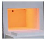
Muffle heated from four sides
