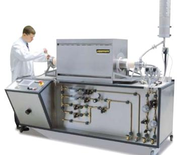
RHTH 120-600/18 with gas supply system 4 for hydrogen operation
