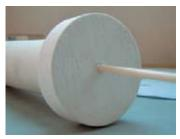
Gas supply system 1: Fibre plugs with protective gas connection, suitable for many laboratory applications
