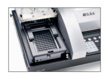
An available vacuum filtration module automates the washing of 96-well filter bottom plates. Vacuum is adjusted via a range of settings for optimal performance with various filter pore sizes.
