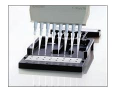
Combined with the Take3 Multi-Volume Plate, the Synergy HT can measure samples down to  $2~\mu L$ .
