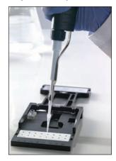
Use Take3 for 2 µL sample measurements in BioTek's Epoch, PowerWave™ XS2 or Synergy™ Multi-Mode Microplate Readers. The precision printed, fused silica slides are easy to pipette onto...and clean up is simple - just wipe with a laboratory tissue.
