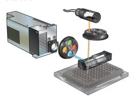
The combination of deep blocking interference filters and dichroic mirrors provides very high performance in all fluorescence read modes (fluorescence intensity, fluorescence polarization, time-resolved fluorescence, AlphaScreen/AlphaLISA).
