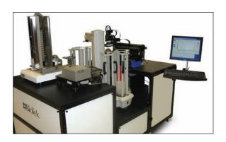
To automate an avian influenza assay for poultry testing, a BioStack Twister II system was designed incorporating 1 Precision™ XS Pipetting System, 3 MicroFill™ Dispensers, 1 ELx405™ Washer, 1 PowerWave™ Spectrophotometer and 1 LiCONic Instruments Plate Hotel.
