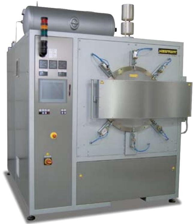
NR 200/11 H<sub>2</sub> for heat treatment under hydrogen
