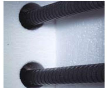
Furnace chamber with high-quality fibre materials and SiC heating rods on both sides of the furnace
