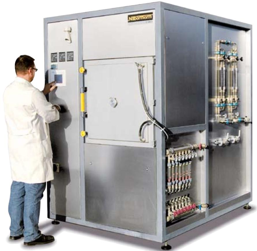
VHT 40/22-GR with graphite insulation and heating
