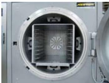
Process chamber with internal heating
