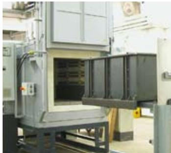
Debinding under protective gas with a gas box in a chamber furnace
