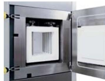
Ceramic fiber heating chamber
