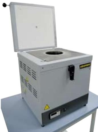
K 2/10 with steel crucible for lead melting
