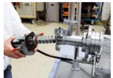
Screw conveyor with adjustable rotational speed
