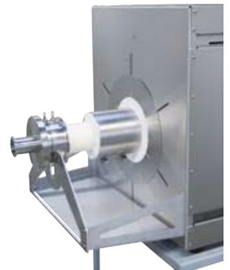
Gas-tight design with water-cooled flanges
