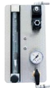
Gas supply panel for nonflammable protective gas with shutoff valve and flow meter with regulator valve, piped and ready to connect
