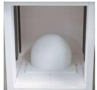
Gastight retort with gas injection through the furnace floor
