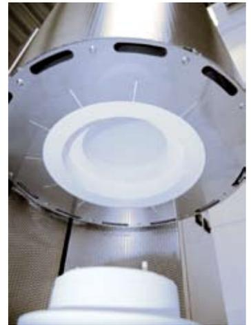
Plasma ceramic retort for protection of the heating elements and to avoid charge continuation [in the LHT 02/16 LBR]
