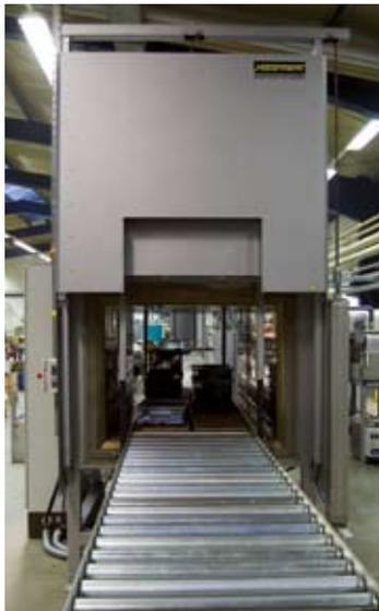
N 1680/45 AS with roller conveyor implemented in a production line
