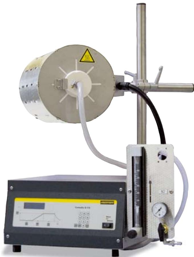
RT 50-250/11 with gas supply system for nitrogen
