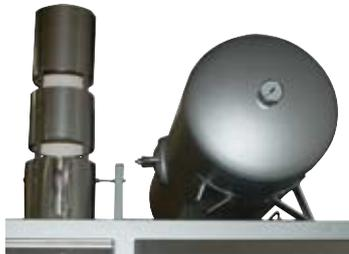
Emergency flood container and exhaust gas torch for model NRA 150/11 H<sub>2</sub>
