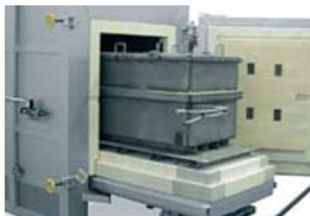
Debinding under protective with a gas box in a bogie hearth furnace
