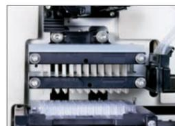
BioTek's patented Dual-Action manifolds provide independent control of aspirate and dispense functions.
