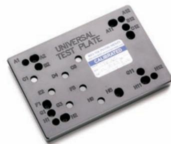
BioTek's Absorbance Test Plate is a convenient tool for GMP/GLP compliance. Fast and easy testing of the ELx800's optical system allows for worry-free, uninterrupted operation. Use on the ELx800 alone, or through the Gen5 Data Analysis Software diagnostic interface for reporting and results archiving.
