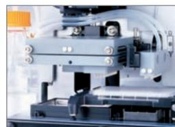
1536-well microplates are washed with two 32-tube manifolds and one 128-tube aspiration manifold for speed and efficiency.
