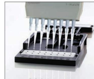
Combined with the Take3 Multi-Volume Plate, the Synergy HT can measure samples down to 2 µL.
