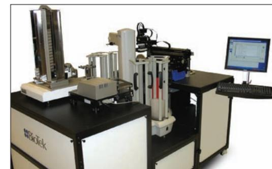
To automate an avian influenza assay for poultry testing, a BioStack Twister II system was designed incorporating 1 Precision™ XS Pipetting System, 3 MicroFill™ Dispensers, 1 ELx405™ Washer, 1 PowerWave™ Spectrophotometer and 1 LiCONic Instruments Plate Hotel.
