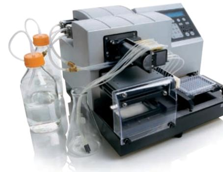
The only instrument on the market offering fast microplate washing along with both peristaltic and microprocessor-controlled syringe drive reagent dispenser technologies to optimize liquid handling processes in the microplate format, including complex wash routines.
