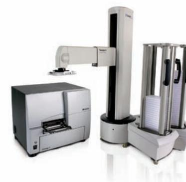
Synergy 2 is easily integrated into robotic systems, and has been validated with all major screening detection technologies including TR-FRET, fluorescence polarization, and AlphaScreen.
