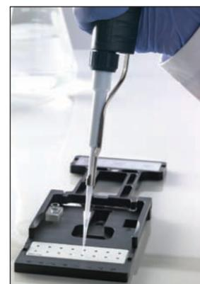
Use Take3 for 2  $\mu$ L sample measurements in BioTek's Epoch, PowerWave™ XS2 or Synergy™ Multi-Mode Microplate Readers. The precision printed, fused silica slides are easy to pipette onto...and clean up is simple - just wipe with a laboratory tissue.
