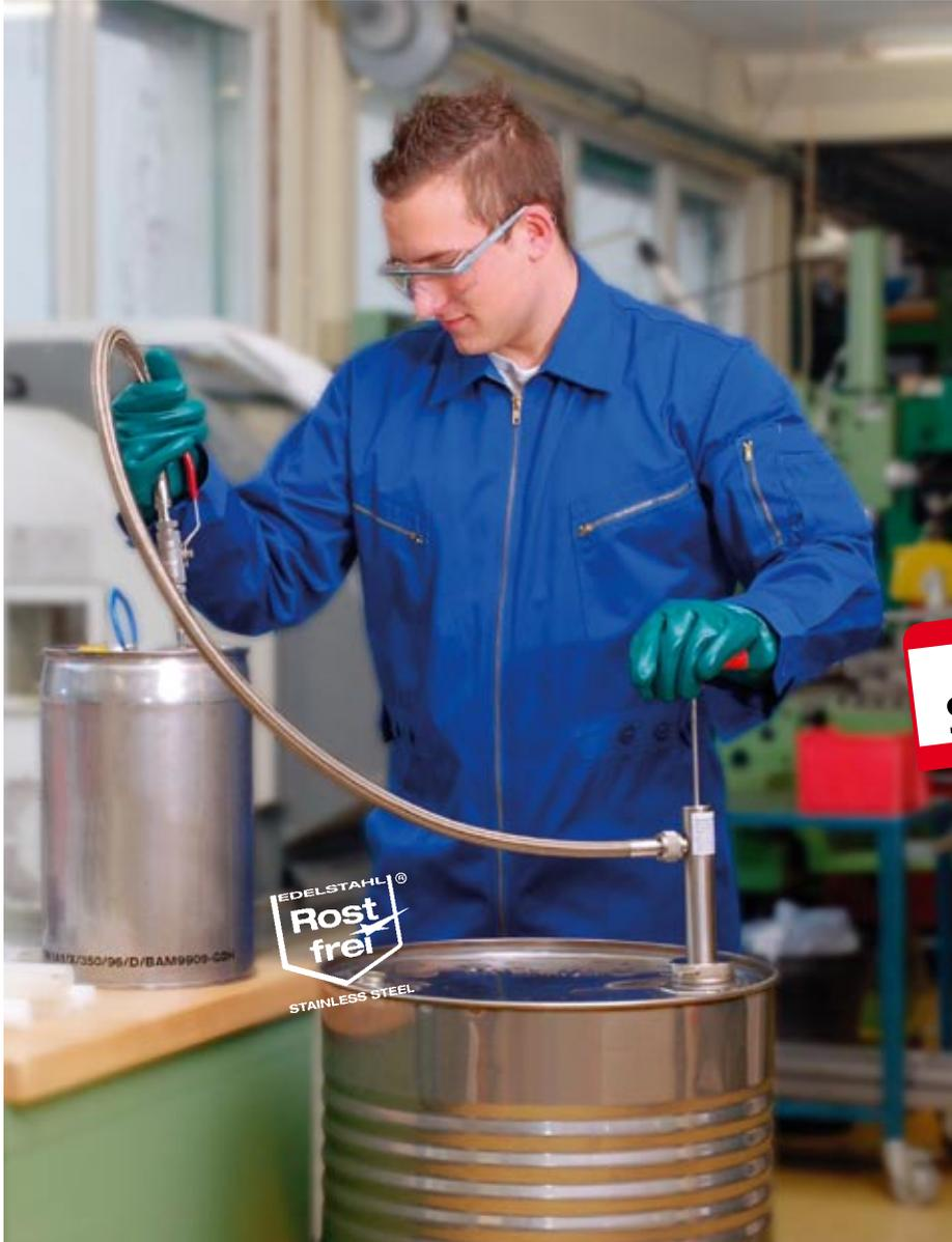
The Bürkle barrel pump made of stainless steel is constructed for filling combustible and easily inflammable liquids. The pump can conduct electricity and consequently fulfills the requirements for handling flammable liquids in combination with the accessory antistatic set.
