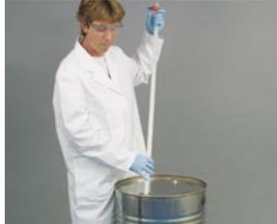
Made of PP for rapid and simple spot checks of liquids. The dip samplers are transparent and enable the contents to be seen clearly. Upper end with reflux valve, lower end with ball valve.
