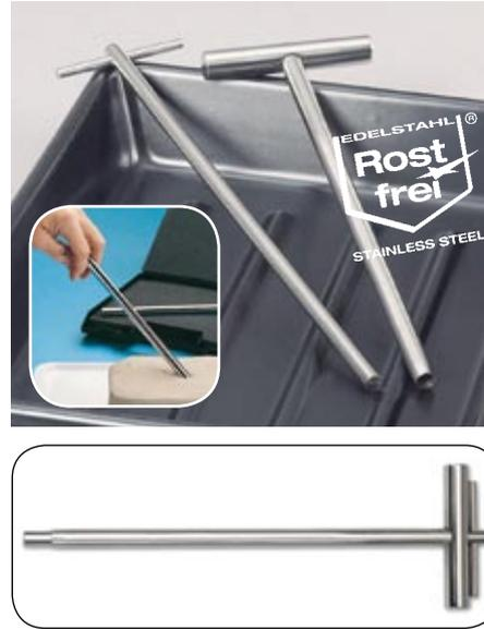
Cylindrical hollow drill with a sharp cutting edge. The hand-drill can easily be driven into paste-like and semi-solid substances by a rotating movement. The samples cut out are subsequently removed from the drill using the push-rod ejector. Drilling depth 20 cm, total length 260 mm, weight 386 g. Inside diameter 8 mm, Outside diameter 10 mm.
