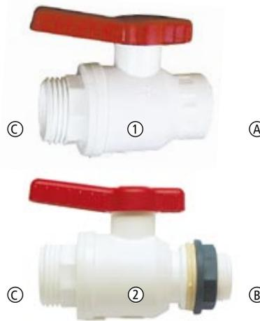
New – now also for foodstuff, made of fibre-glass reinforced PP, ball made of PP-G, handle with O-ring NBR, seal HDPE. Max. pressure 10 bar (at + 20 °C), max. temperature 100 °C. Inner thread
