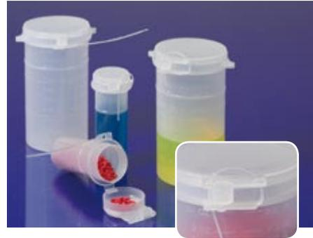
The sample tubes are produced under clean room conditions and formed at over 100 °C in the injection molding machine, so that the insides of the tubes are virtually sterile. This method makes the tubes absolutely leak-proof, as the cap and tube adapt optimally to each other during the cooling process. Undercut-free, so easy to fill and can be emptied completely. With seal guaranteeing virtual sterility until first-time opening.
