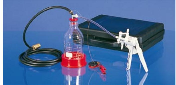
Developed for sampling flammable liquids of hazardous materials VbF Hazard Class A1 (VbF is the German Regulation concerning Flammable Liquids). Glass bottle and hose are connected in such a way that they conduct electricity and are grounded via a grounding cable.
