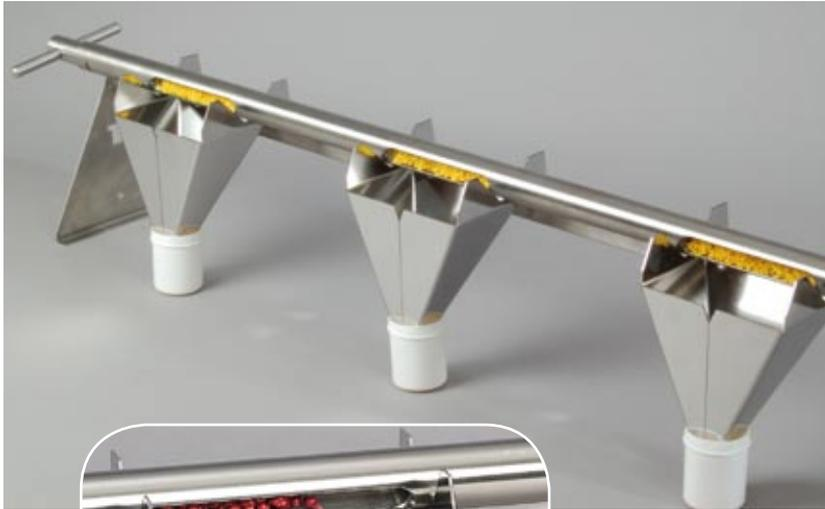
Take a sample, place the zone sampler on the emptying device, push the funnel to the height of the collecting chamber, place the sample container (e.g. 6214-0060, see page 136) beneath it, turn the zone collector with its chamber open – ready!
