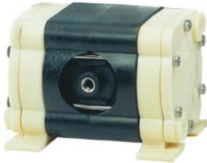
Oil-free Double-diaphragm pumps operated by compressed air offer the solution for transferring viscous, corrosive, abrasive and flammable liquids. Pump version 1/4" (larger pumps available on request). Pump versions made of polypropylene (PP), PVDF and PA are available.
