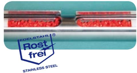
Special sampler for powders and granules that do not flow freely. The sample is transferred to the closable inner tube using a scraper. Sliding PTFE separators are used to divide the inner tube into different zones. The separators also prevent the sample from being mixed.
