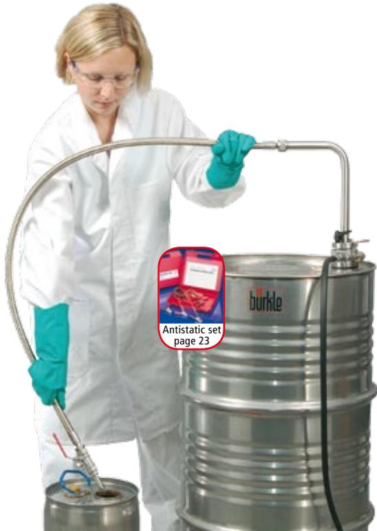
For filling off high-purity liquids. All parts coming into contact with the media are made of stainless steel and FPM (Viton). The barrel screw joint and stopcock provide a hermetic seal between the container and the pump so that unwanted vapors cannot escape during the filling process. Massive, long-life industrial version.
