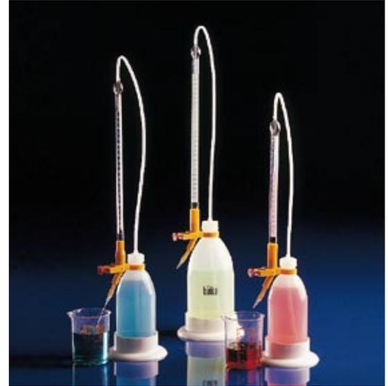
A universal aid in the laboratory, electroplating industry, for field analyses, in water treatment plants, etc. Easy dosing is achieved with the press button, fine titration with the micro-screw and precise discharge jet.
