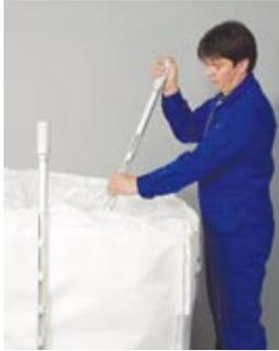
Ensures accurate zone sampling from all layers of the bulk goods. The spiral arrangement of the sampling slits means that these are opened one after the other from bottom to top. In this way the lowest opening is filled first and then those above it in sequence until the complete Spiralus has been filled. The shape of the sampling slits prevents seeds from being cut up,
