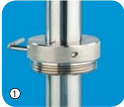
**Brass barrel screw joint** for barrel pumps made of stainless steel. Prevents electrostatic charges in connection with the anti-static set. For safe decanting of flammable and hazardous liquids. For containers with internal R2" steel barrel thread.
