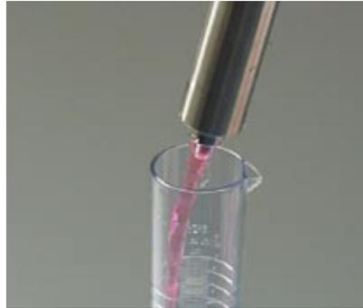
Liquid-Sampler for single hand operation. The valve is opened and closed using your thumb for type 1 or semi-automatically for type 2. Made of AISI 304 stainless steel.
