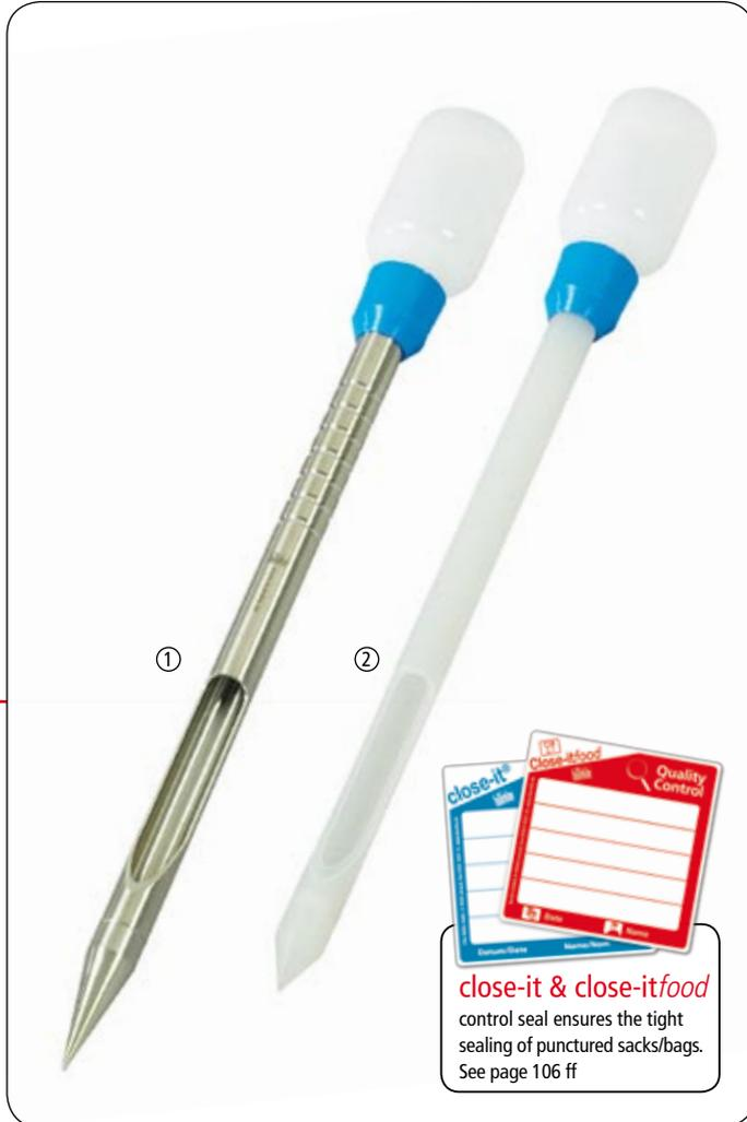
Particularly suitable for taking direct samples of bulk goods from sacks, Big-Bags or open containers and then filling them directly into original sample bottles. QuickPicker is uncomplicated to use and clean. No undercuts or edges mean no sample residues which could falsify subsequent samples. QuickPicker is delivered complete with 2 sample bottles and cleaning brush.
