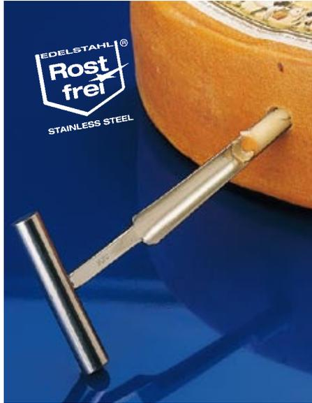
Conical hand-drill, conically shaped, with sharp cutting edges and a solid handle. For taking samples from soft, paste-like substances (cheese, butter, soap, wax, etc.).
