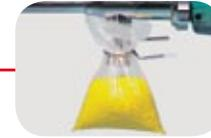
The sample bag is attached to the lance with a clip.
