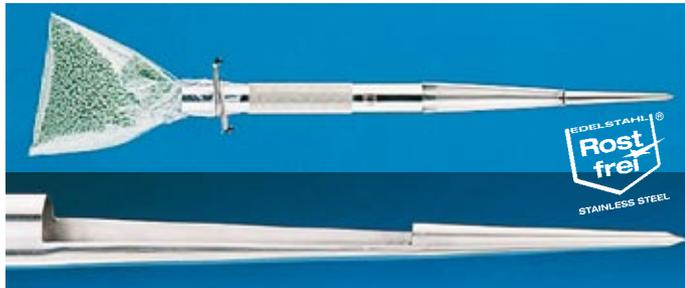
StickProof sampler for powders in the pharmaceutical industry, made of AISI 316 stainless steel. The especially slender tip can be inserted easily and deeply. The conical inlet of the tip lets you collect either very small or larger quantities. StickProof is constructed in one piece without edges, grooves or crevices for perfect and easy cleaning. The sample can be filled directly into the sampling bag. Fasten the bag with a sturdy clamp.
