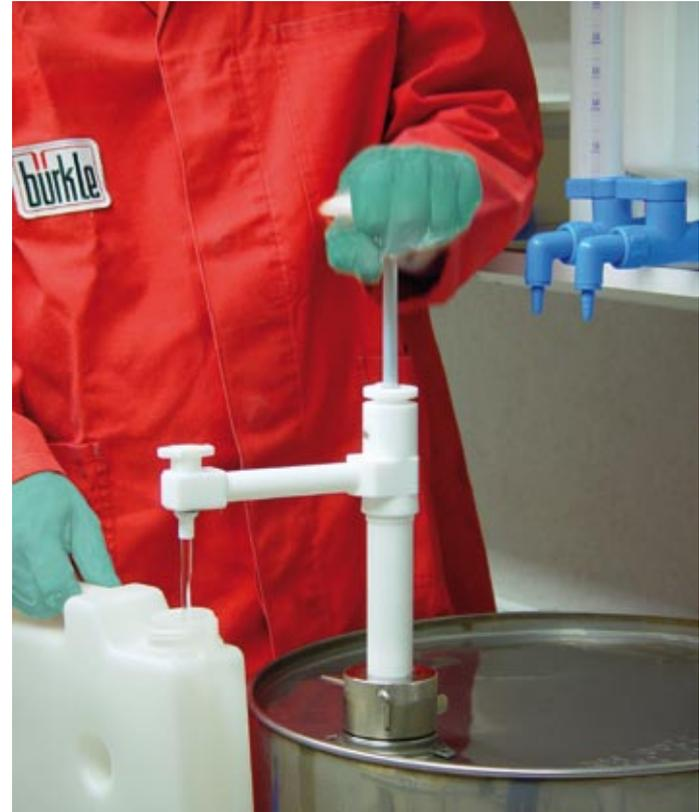
For transferring ultrapure liquids. Liquid-contacting parts made of PTFE and FEP, with their chemical resistance even liquids which attack conventional materials such as PP or PVC can now be safely transferred (except for elemental fluorine). The stopcock prevents hazardous vapors from escaping and stops dripping.
