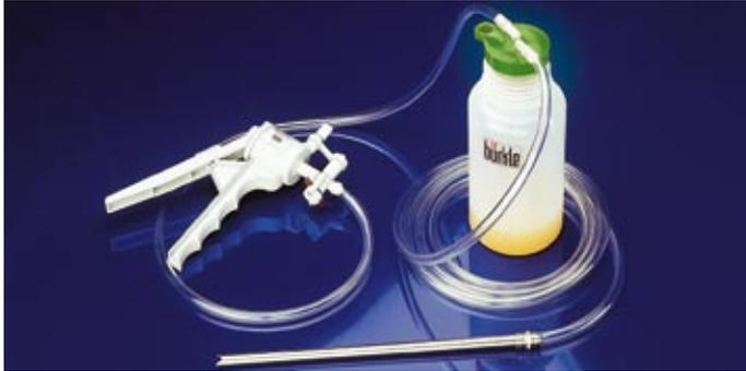
UniSampler with hose and hose weight made of stainless steel. Sampler for deep, narrow and hard-to-reach spots. The heavy stainless-steel tube brings the hose to any desired depth. The samples are also collected using a hand-operated vacuum pump and transferred directly into the sampling bottle to ensure sampling purity.
