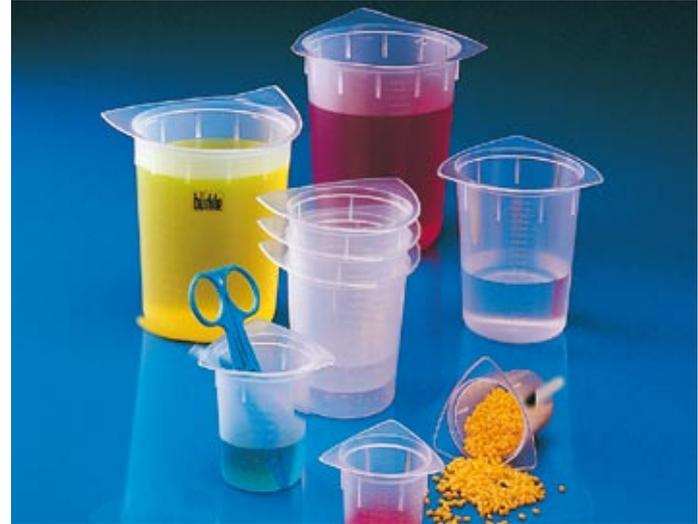
Universal disposable graduated beakers with indestructible graduation. The 3 dimpled spouts enable the safe pouring of liquids.
