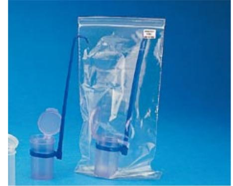
For sterile sampling of liquids or powders. The sample is collected directly in the sampling container and sent for analysis. Prevents cross-contamination.
