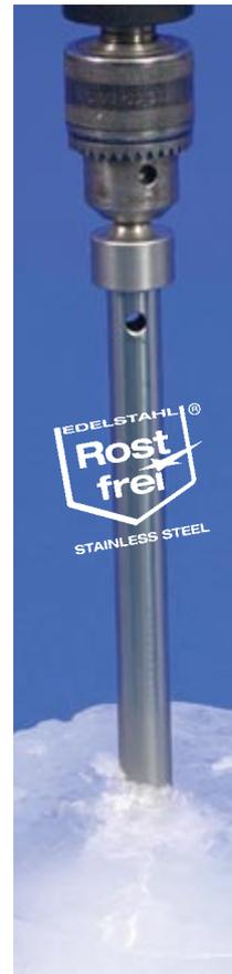
For deep-frozen products in the food industry and semi-solid substances. The sharp sawing crown of the very robust hollow borer rapidly cuts into the sample. A cylindrical sample (cross-sectional sample) with a diameter of 18 mm and a length of up to 20 cm can be cut out. Consists of three parts: borer, borer head for use in conventional drills and rod for pressing the cylindrical sample out of the borer head.
