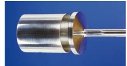
Collects liquids of varying viscosity. Media containing particles can also be sampled without difficulty. The sampler can be used in the fields of chemistry, foodstuffs and cosmetics. The cup can be unscrewed from the stem, allowing easy cleaning. Made completely of AISI 316 stainless steel.
