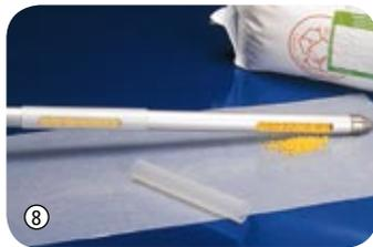
⑧ Sealing sleeves in PP, sterilizable, used to close individual chambers when filling, emptying or transporting 25 mm dia. zone samplers. The sealing sleeves are easy to slide on and automatically clip into position. Length 150 mm.
