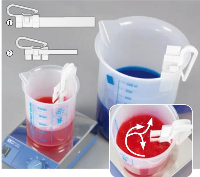
When agitating with magnet or overhead agitators, usually a laminar current with little turbulence tendency develops. Baffle clips disturb the flow direction and provide a substantially better mixing of the liquid in such a way. Baffle clips are made of PP. They come with two differently large and exchangeable blades, which fit in beakers from 1 l to 5 l.
