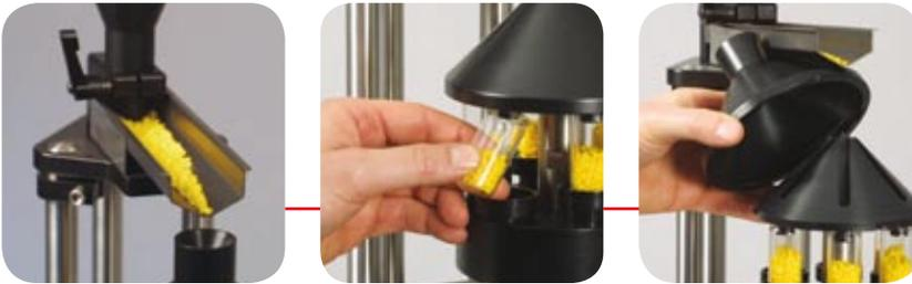
Distributor head for sample tubes with different shapes and sizes
