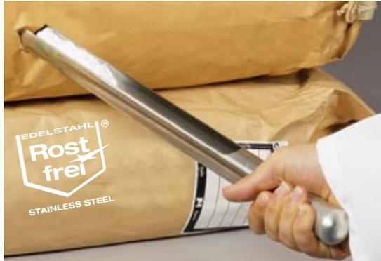
Milk powder collector made of AISI 316 stainless steel, sterilizable. Developed especially for milk powder samples, conforms to standards of DIN and IDF (Int. Dairy Federation). The collector is inserted into bags or casks and the sample is removed using a semi-circular profile lance.
