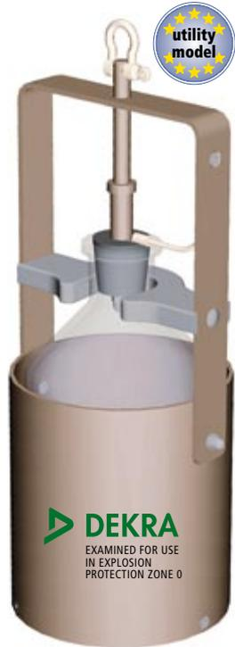
For taking sludge and water samples in sewage treatment plants. For testing crude oil, liquid petrochemicals, fuels, special and test benzene, fuel oils, kerosene and liquid lubricants of Hazard Classes AI and AII (VbF). Completely made from non-spark-producing materials. Dipping frame made from nickel-plated brass, Easy-Click closure made from electrically conductive polyamide. Suitable for use in Ex-proof areas (observe the safety regulations)!
