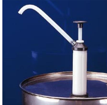
The piston pump is made of polypropylene and polyethylene, for aqueous and petrochemical products. It offers a good price/performance ratio. The piston pump is attached to the container with a 2" or 3/4" internal thread connection. After mounting it can still be rotated about its axis so that containers can be placed on the drum lid and filled.
