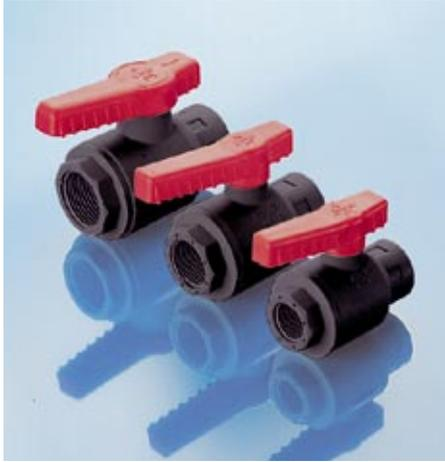
Made of fibre-glass reinforced PP, red handle with Viton and PTFE O-rings, maximum pressure 10 bar (at + 20 °C), maximum temperature + 100 °C.
