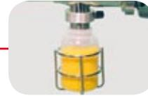
The **bottle basket** is used to attach a sample bottle to the lance.
